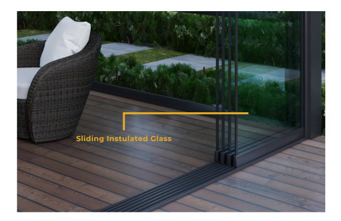
The Sliding Glass System consists of horizontally sliding panels. Depending on the profile type, the system uses 5/16" (8mm) tempered glass or 5/32+15/32+5/32" (4+12+4 mm) tempered insulated glass units.
